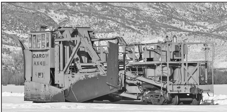
D&RGW Jordan spreader AX45 was in the yard at Phippsburg, Colorado, on January 21, 2015. It was the last piece of snow fighting equipment that the Rio Grande bought before the mergers. – Photo © 2015 Dave Schaaf.
