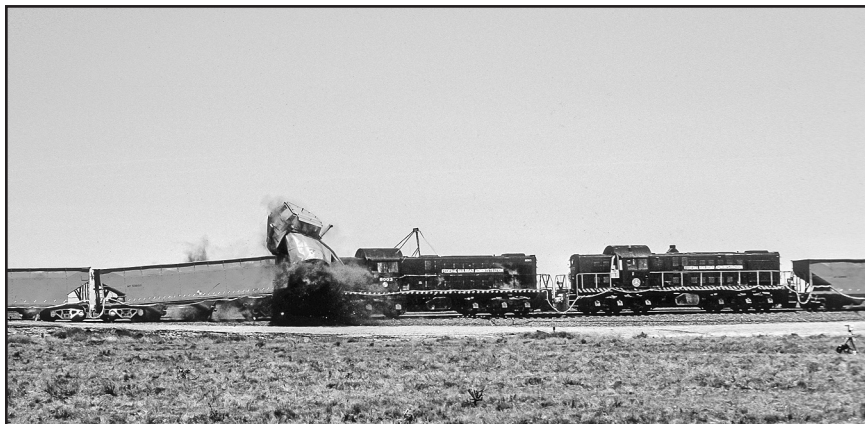
This Department Of Transportation image is from a series of crash tests during 1975 to validate the crash-worthiness computer logic used in cab design and evaluation. – Photo © 1975 Bruce Barrett.
